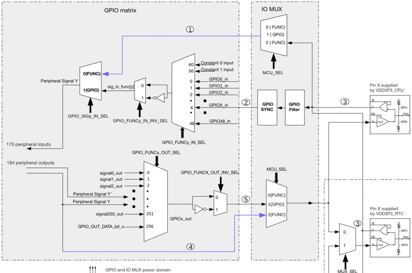
IO MUX pin settings (selected function, drive strength, pull-up, pull-down, input enable) are controlled by the children of the `iomux`: `pinctrl@60009000` node, like this:
